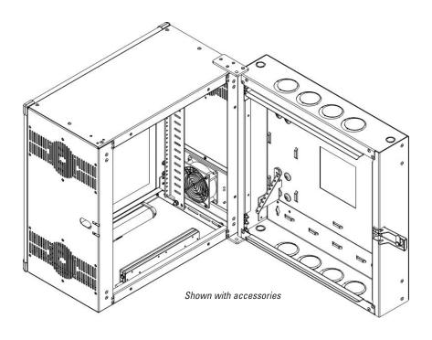
One pair of mounting rails with EIA-310 compliant universal 5/8"-5/8"-1/2" alternating hole pattern are included with each cabinet and are fully adjustable front-to-rear
