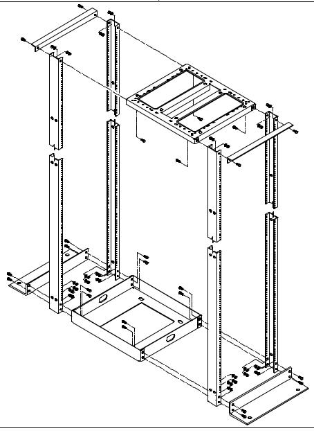
The new QuadraRack 4—Post Kit is designed to easily build a high capacity 4—Post Frame.
