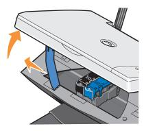
The ink cartridge carrier moves and stops at the loading position unless the printer is busy.
