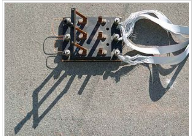
Triple-pole single-throw (TPST or 3PST) knife switch used to short the windings of a 3-phase wind turbine for braking purposes. Here the switch is shown in the open position.
