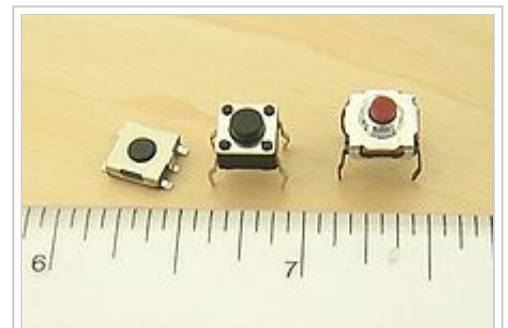
Three push button switches (Tactile Switches). Major scale is inches.
