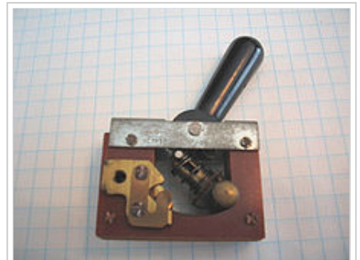
Large toggle switch, depicted in circuit "open" position, electrical contacts to left; background is 1/4" square graph paper
