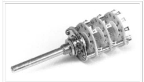
A three-deck stacked rotary switch. Any number of switching elements may be stacked in this manner, by using a longer shaft and additional spacing standoffs between each switching element.
