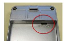
Auto Shut-Off Enabled = ON Auto Shut-Off Disabled = OFF
