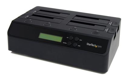
The SATDOCK4U3RE USB 3.0 and eSATA 1-to-3 Hard Drive Duplicator docking station enables you to duplicate/clone a single SATA hard drive to up to three other SATA drives simultaneously, as a standalone device. The duplicator can also function as a regular 4-bay hard drive docking station, by connecting to a host computer system.
