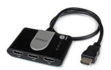
The VS123HD 3-port HDM® Auto Switch features three prioritized HDMI input ports. If the active HDMI source is turned off, disconnected, or otherwise lost, the switch automatically selects the next available HDMI signal as the priority output, ensuring the display is always receiving a signal.
